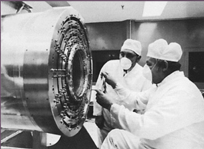
Nested “mirrors” of Chandra X-ray telescope
