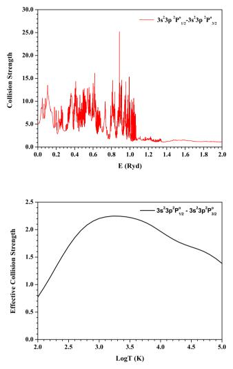
**Figure 2.** (a) Collision strength for the 17.9  $\mu$ m [P III] IR fine structure transition. High resolution at near-threshold energies is necessary for accuracy in rate coefficients at low temperatures. (b) Maxwellian averaged effective collision strengths  $\Upsilon(T_e)$  (equation 5). There is a factor of 3 or more variation broadly peaking at typical nebular temperatures  $T_e > 10^3$  K. structures.
