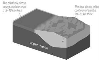
Plates float on a complex transition zone where basaltic lavas form.
