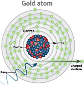
When an X-ray with a specific wavelength strikes a gold atom, it kicks out an inner electron. An electron on a higher energy level then falls to fill its place, emitting an X-ray and electron in the process. If scientists place a gold nanoparticle into a cancerous tumor, this process could destroy the cancer by flooding it with radiation and electrons. Astronomy: Roen Kelly
