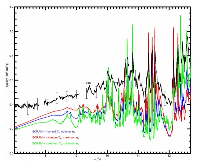
Extended Data Figure 5 | Evaluation of changes in the model-data comparisons at the error bounds determined for the plasma conditions. The measured iron opacity at  $T_e = 2.11 \times 10^6$  K and  $n_e = 3.1 \times 10^{22}$  cm<sup>-3</sup> is denoted with a black line, with error bars corresponding to the  $1\sigma$  uncertainty.
