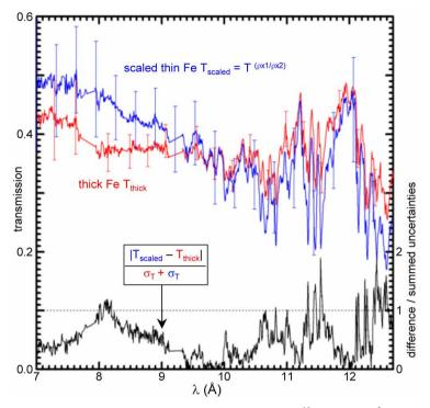
**Extended Data Figure 4** | **Beer–Lambert–Bouguer scaling test for Be-tamped iron opacity data.** The transmission should scale according to  $T_2 = T_1^{Nx2/Nx1}$ , where Nx1 and Nx2 are areal densities associated with transmissions  $T_1$  and  $T_2$ . The thick iron sample transmission  $T_{\text{thick}}$  ( $NX \approx 1.91 \times 10^{18}$  atoms per cm<sup>2</sup>) is shown in red (left axis). The average transmission for the two experiments using a thin iron sample
