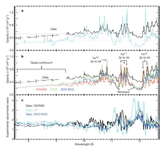
Figure 3 Comparisons of iron opacity spectra with multiple models at the solar radiation/convection zone boundary temperature. The  $T_e = 2.11 \times 10^6$  K,  $n_e = 3.1 \times 10^{22}$  cm<sup>-3</sup> conditions displayed here were deemed to be the most accurate; the opacity represents an average obtained by combining information from five separate experiments with four independent spectrometers. The calculations account for the instrument resolution and
