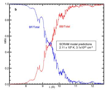
**b**, The SCRAM opacity model predicts that the ratio of the bound–free (BF) opacity contribution with the total opacity (blue) is larger than the ratio of the bound–bound (BB) opacity contribution with the total (red) for wavelengths less than approximately 9.5 Å.
