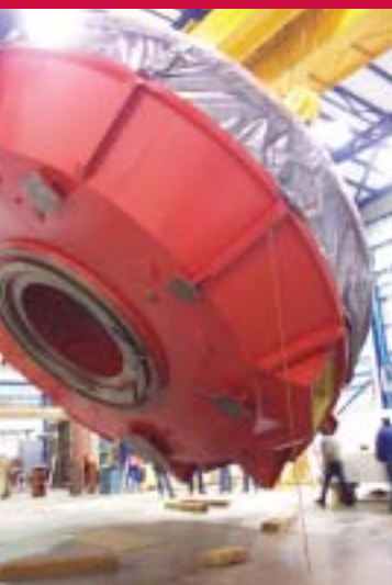
Bottom, integrating the cell with 8.4-meter primary mirror on the left side of the telescope.
