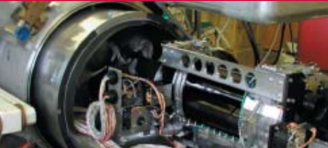
THE INNER WORKINGS OF TIFKAM, AN INFRARED IMAGER/SPECTROMETER AT MDM
