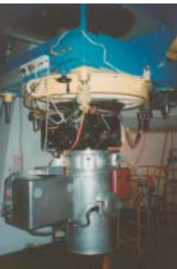
DANDICAM, above, has been deployed at the 1-meter Elizabeth Telescope at the South African Astrophysical Observatory.
