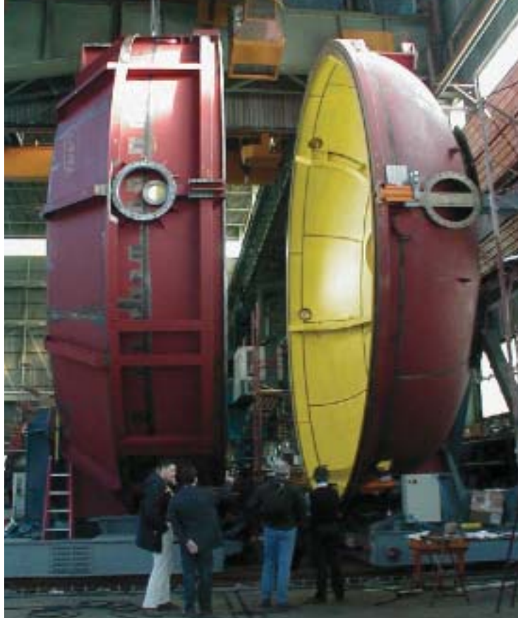
MIRRORS' BELL JAR AND DUMMY MIRROR CELL ON THE TRACK
