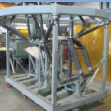
Upper structural frame of the MODS spectrograph under construction at Indian Creek Fabricators, near Dayton, Ohio
