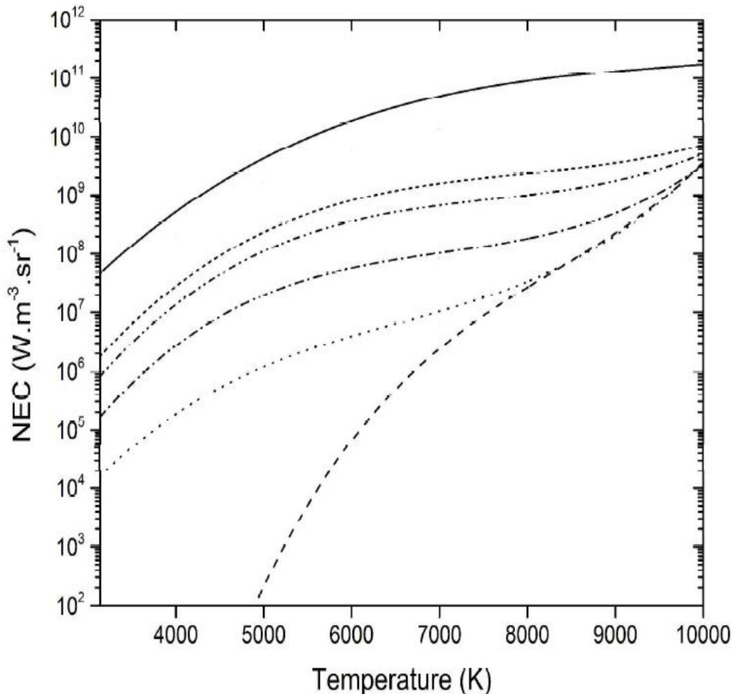
Fig. 6. NEC of nitrogen-iron arc plasma for various iron mole fractions at 0.1 MPa pressure and  $R_p=0$ . Dash line (100% N<sub>2</sub>-0% Fe), dotted line (99.9% N<sub>2</sub>-0.1% Fe), dash dot line (99% N<sub>2</sub>-1% Fe), dash dot dot line (95% N<sub>2</sub>-5% Fe), short dash line (90% N<sub>2</sub>-10% Fe), straight line (0% N<sub>2</sub>-100% Fe).
