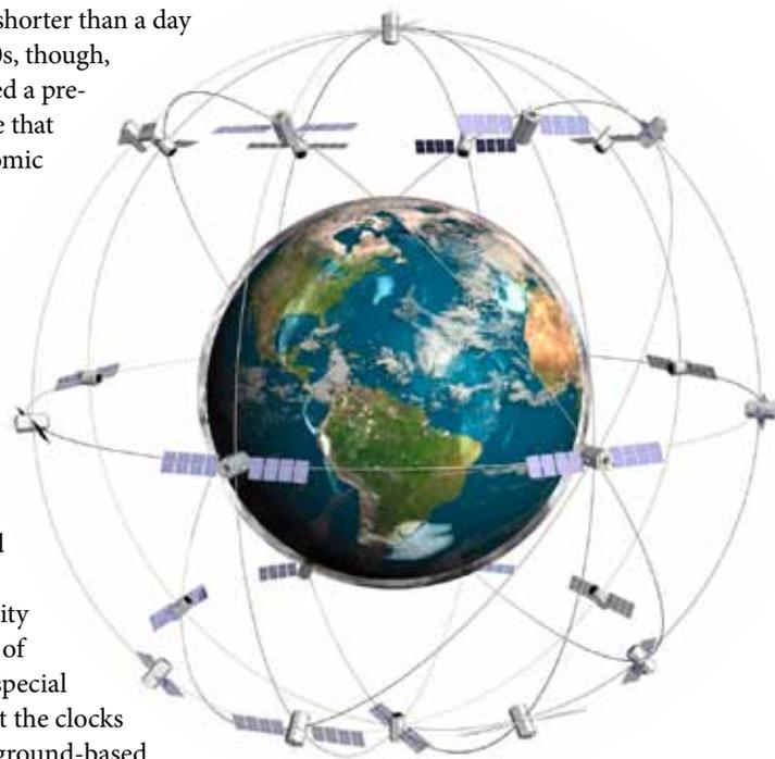
**The Global Positioning System (GPS)** evolved from testing Einstein's relativity theory. While 30 GPS satellites orbit Earth, 24 constitute the navigation system that the public relies on (the other six are backups). © Pixac/Dreamstime.com
