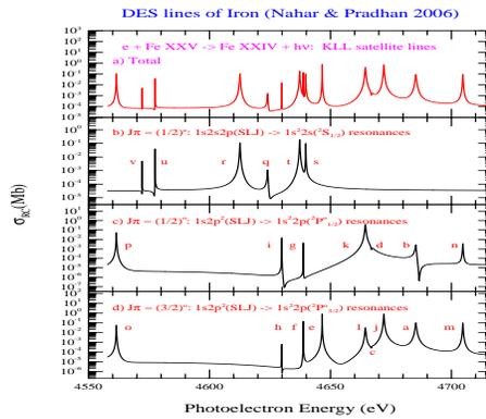
**Fig. 7.** Theoretical study of DES lines, cross sections versus electron energy, seen in solar spectrum [2]. The top panel shows the spectrum that can be observed while the bottom panels identify the component lines, including the overlapped ones, of the total spectrum.
