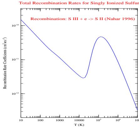
**Fig. 12.** Total recombination rate for singly ionized sulfur, S II, from doubly ionized sulfur S III [5]. The recombination rates shows that starting high at very low temperature it decreases until at a higher temperature where it peaks due to resonances in the process.
