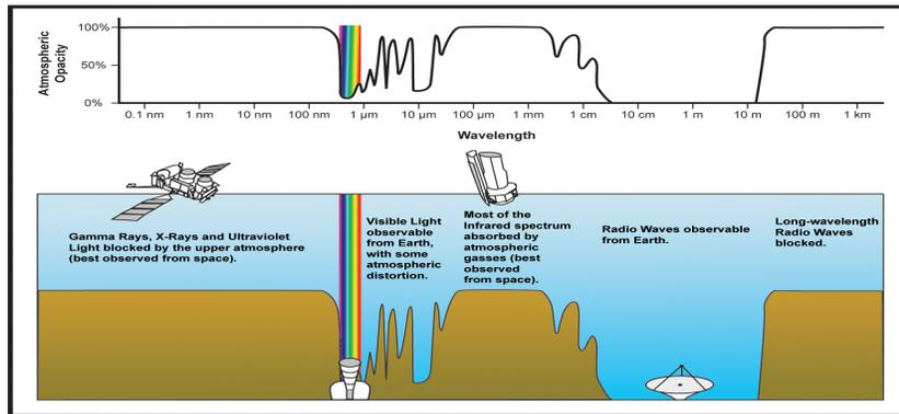
**Fig. 9.** Top: Atmospheric opacity spectrum showing wavelengths ranges of radiation that are blocked by atmosphere due to higher opacity and that reaching the earth due to lower opacity. Bottom: Opacity determines usage of space and ground based telescopes to study the universe. ([www.ipac.caltech.edu/Outreach/Edu](http://www.ipac.caltech.edu/Outreach/Edu))
