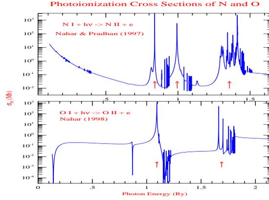
**Fig. 11.** Photoionization cross sections ( $\sigma_{PI}$ ) of oxygen and nitrogen [3, 4]. At energies (pointed by arrows) the resonance peaks indicate enhancement of ionization of the atom by orders of magnitude.
