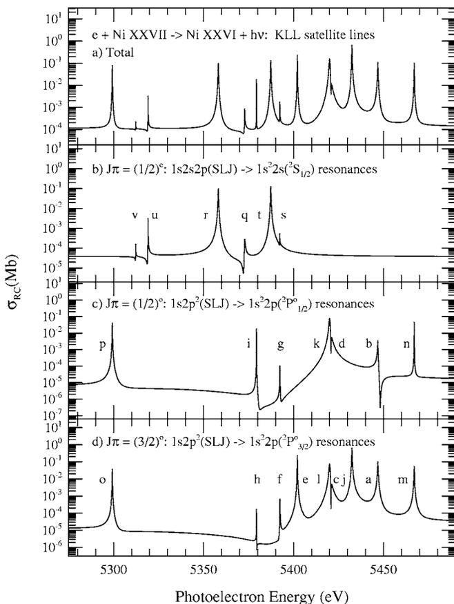
FIG. 2. Satellite lines of Ni xxvii in the  $K\alpha$  complex. The top panel (a) shows the total spectrum and the lower three panels show the resolved and identified lines belonging to final recombined levels (b)  $1s^22s^2(S_{1/2})$ , (c)  $1s^22p^2(P_{1/2}^o)$ , and (d)  $1s^22p^2(P_{3/2}^o)$ .
