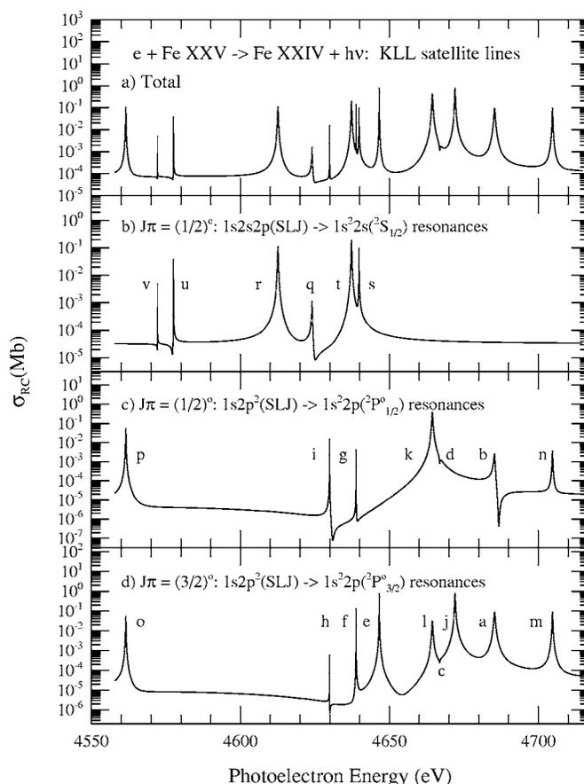
FIG. 1. Satellite lines of Fe xxv in the  $K\alpha$  complex. The top panel (a) shows the total spectrum and the lower three panels show the resolved and identified lines belonging to final recombined level (b)  $1s^22s(^2S_{1/2})$ , (c)  $1s^22p(^2P'_{1/2})$ , and (d)  $1s^22p(^2P'_{3/2})$ .
