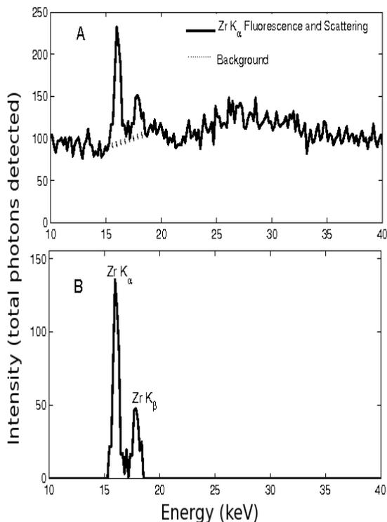
Fig. 8. Production of  $K_\alpha$  X-rays from Zr using 100 keV bremsstrahlung<sup>2</sup>
