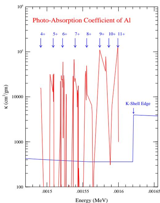
Fig. 9. Resonant  $K_{\alpha}$  absorption coefficients of various ionization states of aluminum, from  $Al^{4+}$  to  $Al^{11+}$ . The background (blue) shows an enhancement at K-shell ionization, however, but much lower than the resonant peaks. Vinko et al.<sup>11</sup> measured enhanced fluorescence at these resonant energies of Al.
