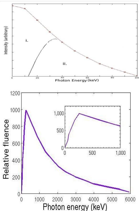
Fig. 6. Bremsstrahlung from a 100 keV (top panel) X-ray source and a 6 MeV LINAC (bottom) with a peak around 35 keV and 300 keV, respectively, after filtering out the lower energy x-rays
