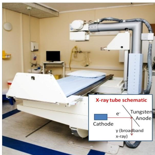
Fig. 5. Typical x-ray machine in a medical facility. The inset shows diagram of production of x-rays
