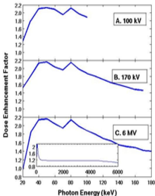
Fig. 4. The radiation dose deposition in tissues for x-ray absorption at three different energies, 100, 170, and 6 MeV from three x-ray sources.
