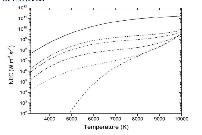
Fig. 6. NEC of nitrogen-iron arc plasma for various iron mole fractions at 0.1 MPa pressure and  $R_v$ =0. Dash line (100%N<sub>2</sub>-0% Fe), dotted line (99.9%N<sub>2</sub>-0.1% Fe), dash dot line (99%N<sub>2</sub>-1% Fe), dash dot dot line (95%N<sub>2</sub>-5% Fe short dash line (90%N<sub>2</sub>-10% Fe), straight line (0%N<sub>2</sub>-100% Fe).
