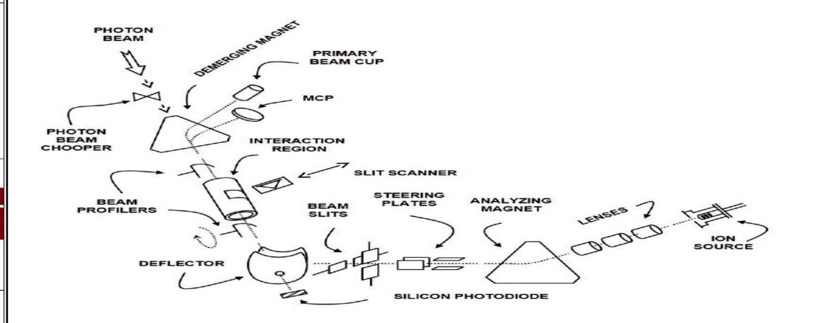
• ALS station for measurement of photoionization cross sections
