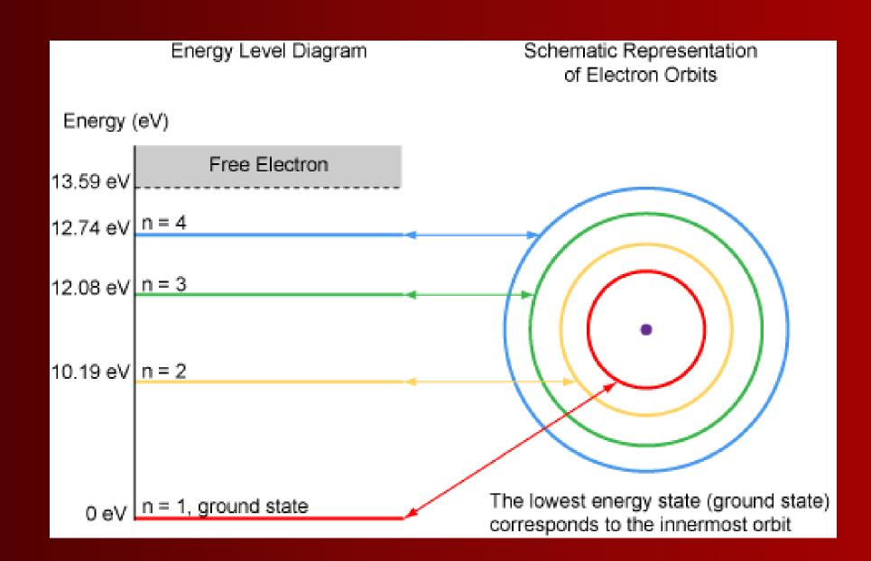
Each orbital corresponds to a quantum energy level as given below:
