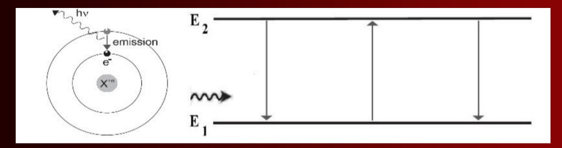
Atomic radiative transition: when an electron goes from one quantum energy level E1 to quantum energy level E2 or comes down from E2 to E1.
