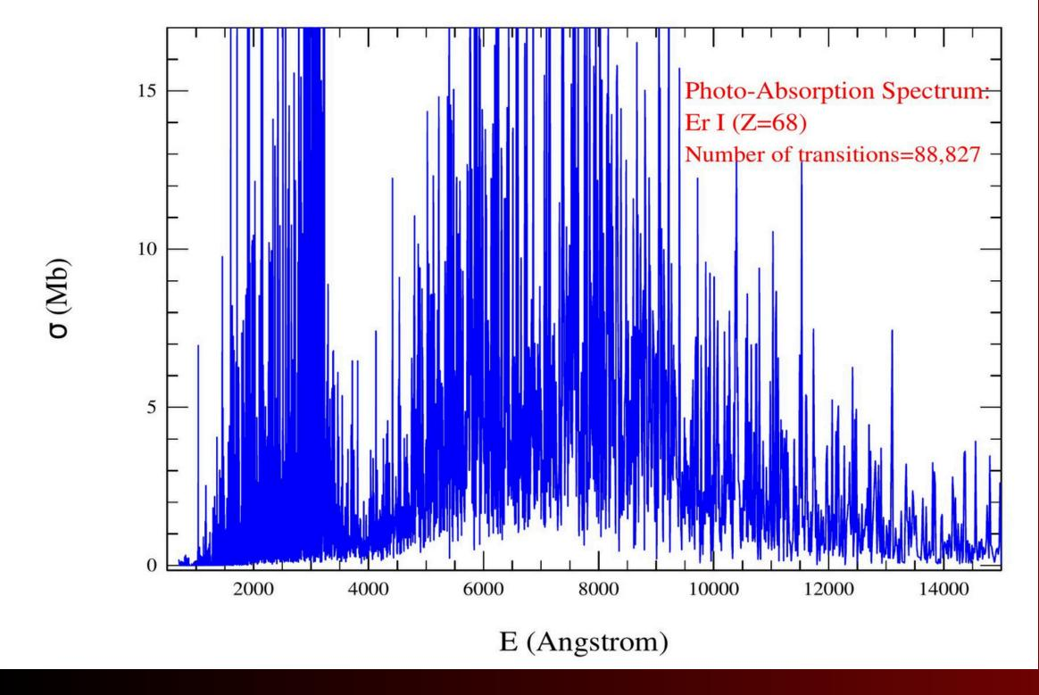
Number of spectralines in this figure is 88,827 making the broad features, the second broad feature is similar to what kilonova produced.
