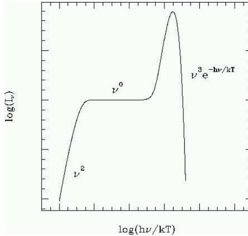
Figure 1: Spectrum of hot gas, showing the effects of saturated inverse Compton scattering at high frequencies.
