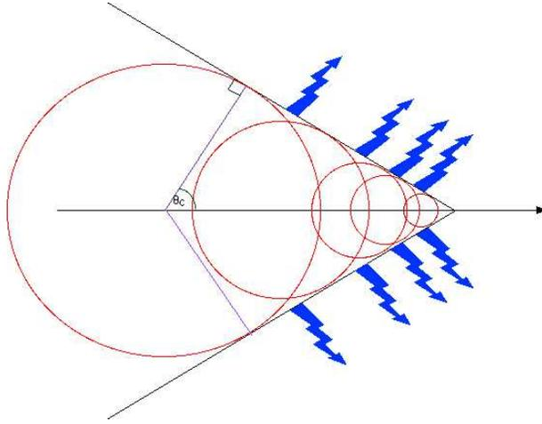
Figure 3: Geometry of Cherenkov radiation.
