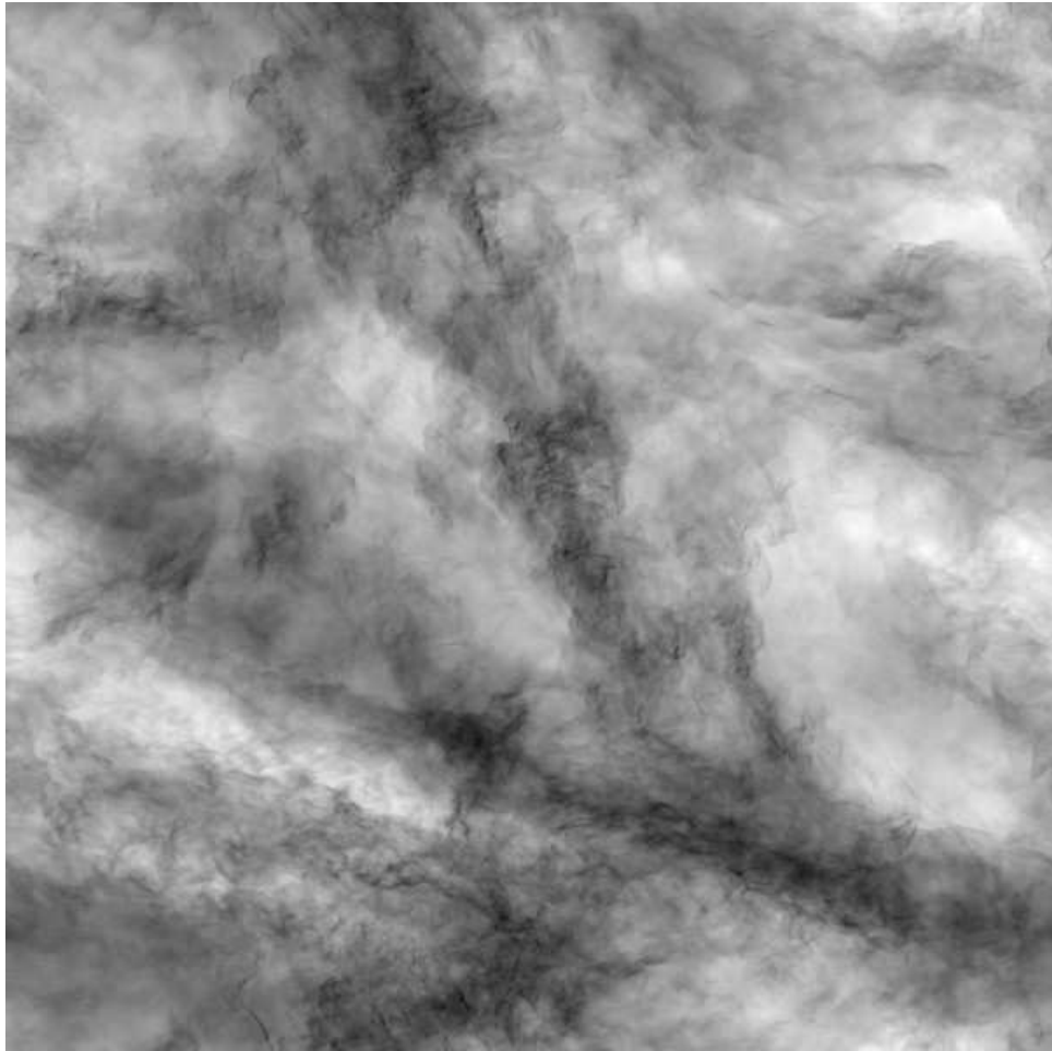
Figure 7.6: Gas density from a 1024^3 adaptive mesh simulation of supersonic compressible turbulence (darker regions are denser). [Kritsuk et al., 2006, ApJ, 638, L25]
